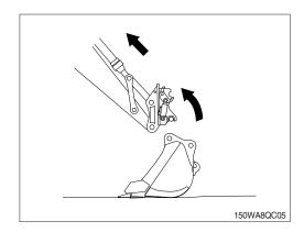
(8) Move the arm (1) and raise it until hook engages the upper (2) pin or interface of attachment.
