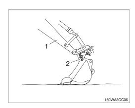
(9) With the bucket crowded, engage the quick coupler to the lower attachment pin or interface.
